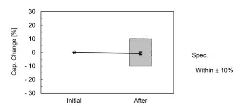
(Dielectric Strength) AC4000V(r.m.s.),60 s and DC6000V,60s Dielectric Strength (Between lead wires) : No failure Dielectric Strength (Body Insulation) : No failure Insulation Resistance (I.R.) :  $1000M\Omega$  min. Appearance : No marked defect
