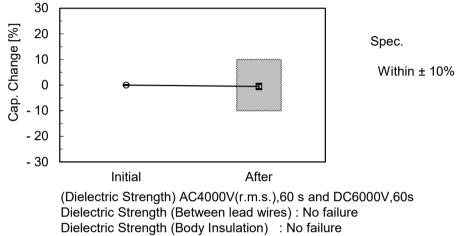
Insulation Resistance (I.R.) :  $1000M\Omega$  min. Appearance : No marked defect
